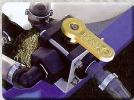
Three-way valve for mixing and circulating the milk.
