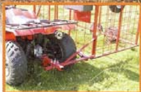
Universal front mount. Hitch mount on rear.
